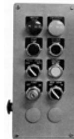
Two cycle-selector switches on the unit's convenient console provide either manual control of all functions or programming by a robot in conjunction with the unit.
