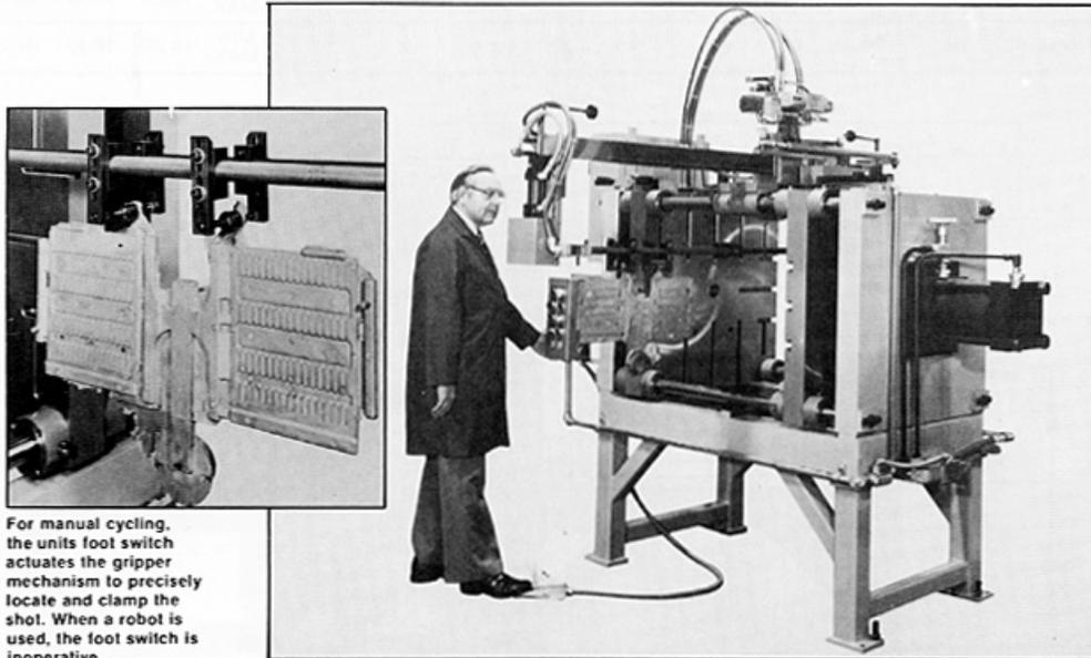
For manual cycling, the unit's foot switch actuates the gripper mechanism to precisely locate and clamp the shot. When a robot is used, the foot switch is inoperative.
